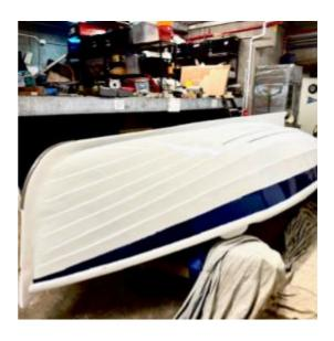
match the original colour. When the treatments are completed, the boat will then be flipped-over to work on the exterior hull, stem, and stern / transom.
